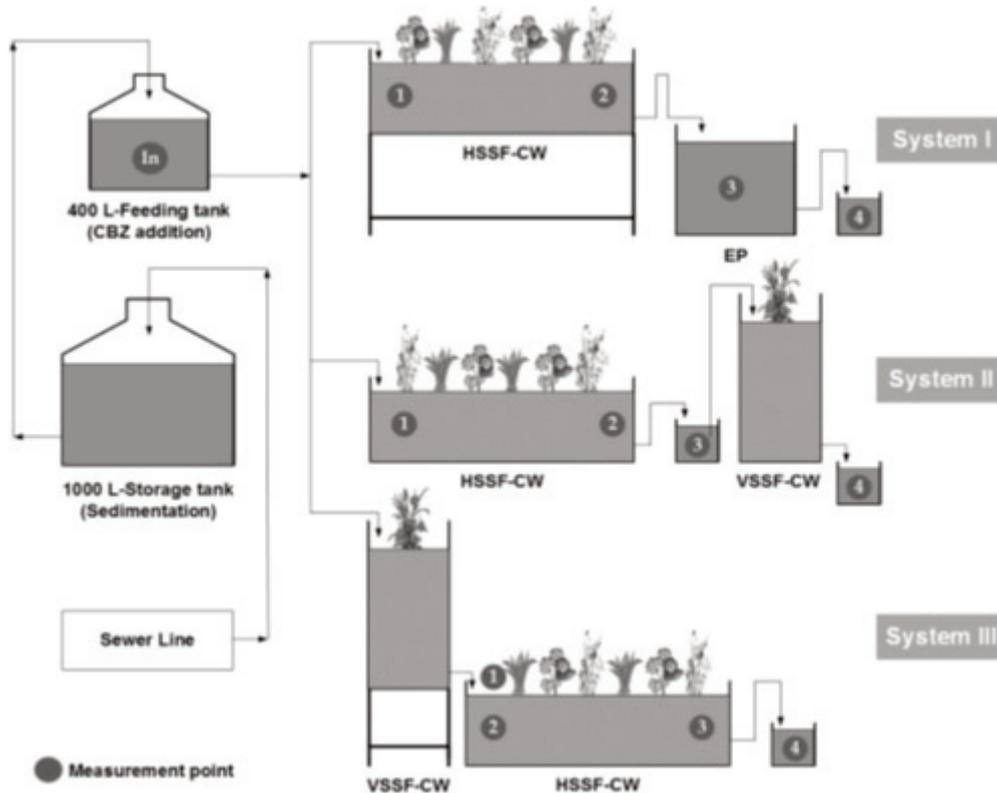
Fig. 1. The hybrid system used for the experiment (Tejeda *et al.*, 2016).
